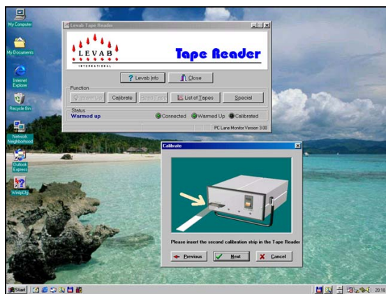
Calibrate the measurement slot of the CLM Tape Reader.
